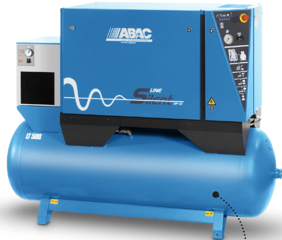
All in one: integrated dryer
